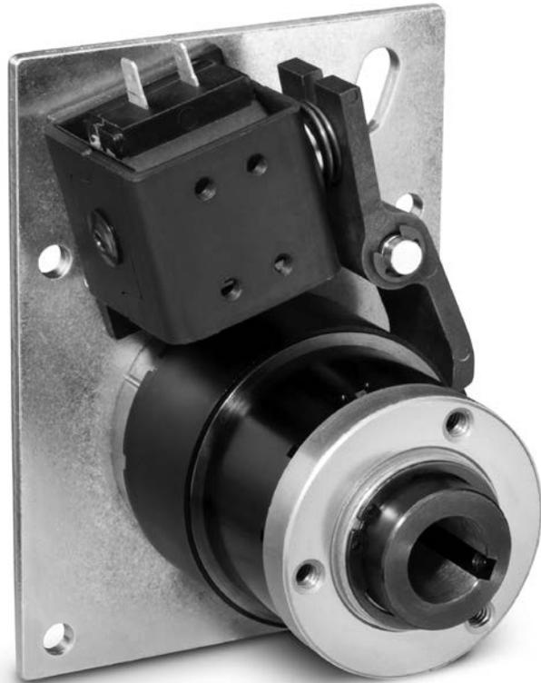
The input hub is drilled and tapped to allow for mounting of sprockets, gears, sheaves, etc. The output is a hollow quill that mounts onto the customer's driven shaft. The backing plate is not a mounting plate. It must be held in place by a loose fit pin to eliminate any side or radial loads from preloading the unit's bearings.
